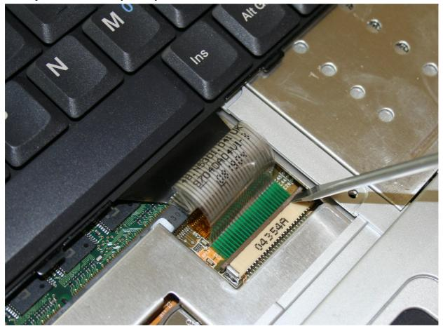
You can now release the cable and remove the keyboard.
