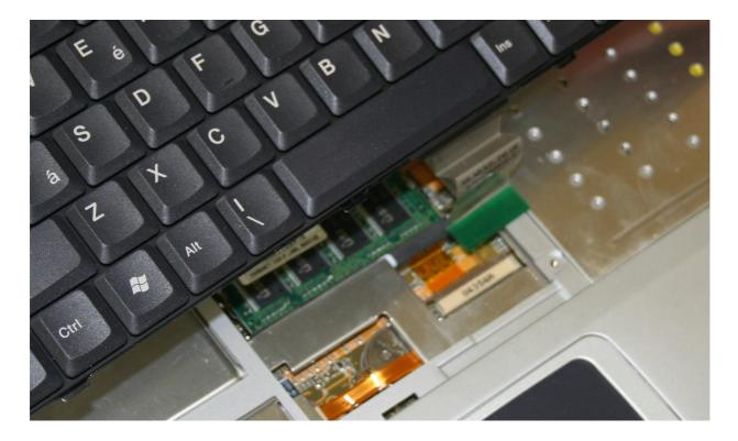
Push the ribbon cable of the new keyboard into the connector so that it is as straight as possible and then gently push the brown clip closed. Reassembly is the reverse of the above procedure.
