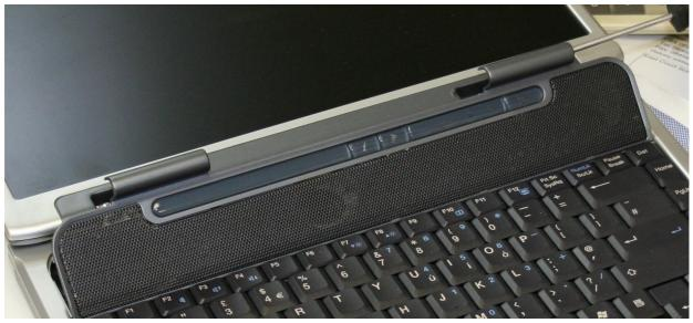
When you have removed the cover plate you will see a small screw at the top of the keyboard in the middle. Using a small Phillips screwdriver remove the screw.
