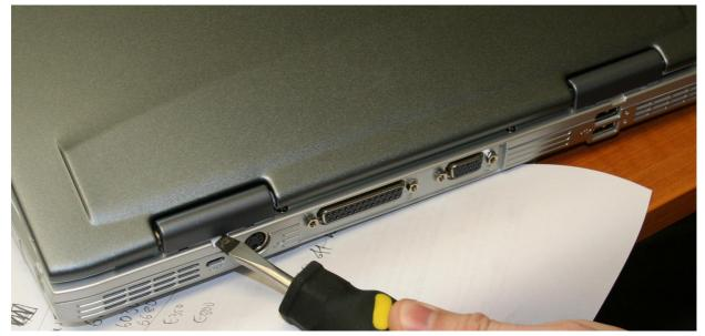
Open the LCD lid and insert a flat blade screwdriver, or preferably a soft tool into it. Give it a gentle twist to unclip it. Do the same thing to the hinge cover at the other end.
