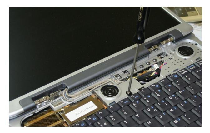
Gently lift the keyboard up and lay it face down on over the track pad. Remove the two screws on the central panel that conceals the ribbon cable connector and then remove the panel to reveal the connector
